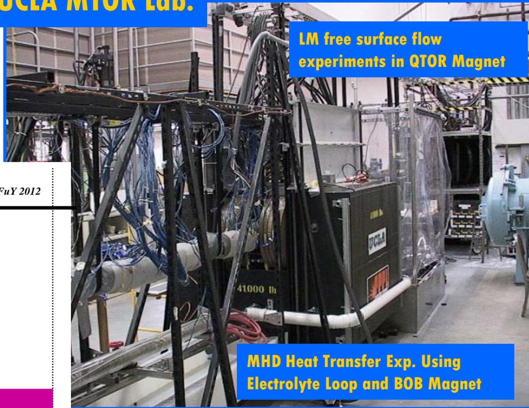
**LM free surface flow experiments in QTOR Magnet**
