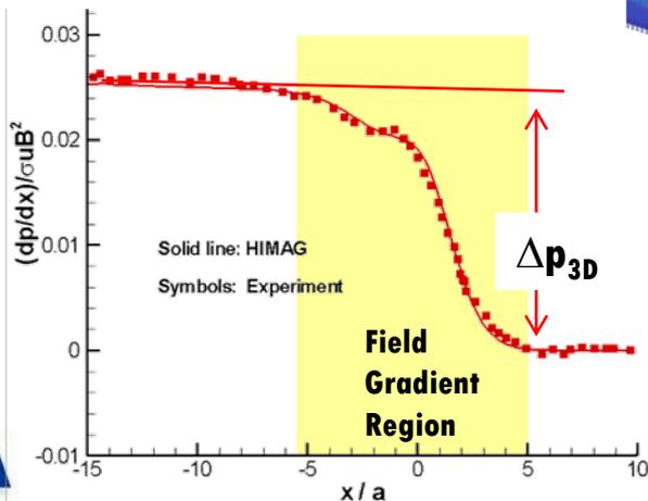
*HIMAG 3D Simulation at  $Ha_{max} = 5000$  in conducting circular pipe*
