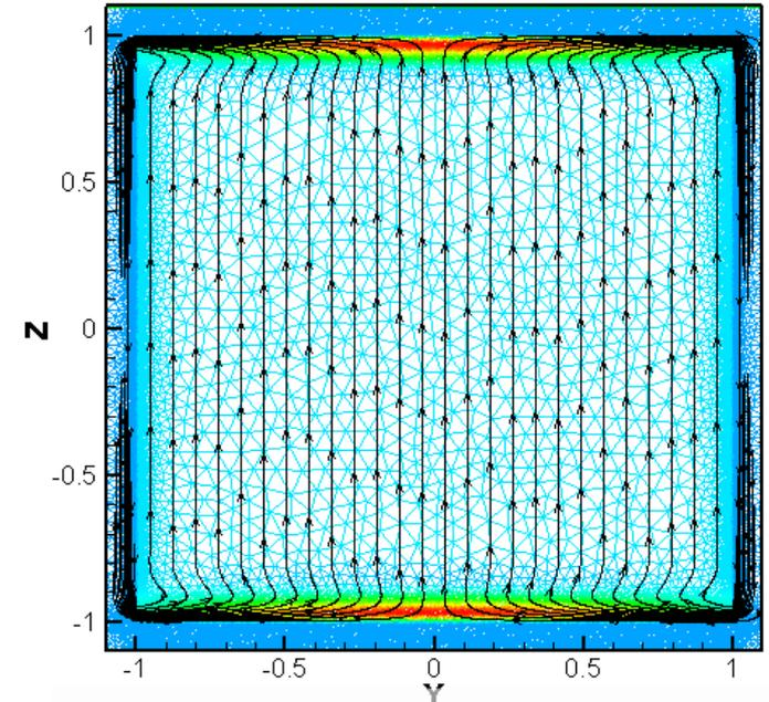
*HIMAG 2D simulation at  $Ha = 1000$  showing good accuracy and current conservation on triangular mesh*
